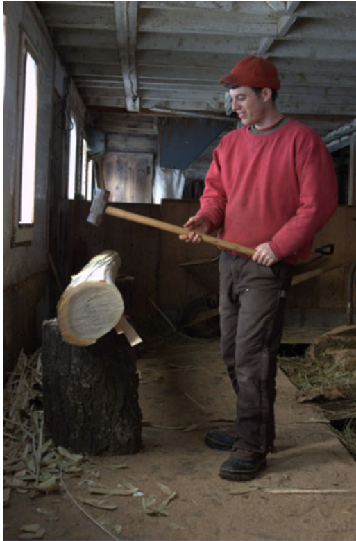
Fig. 1. Pounding black ash logs. Pounding crushes the porous spring growth of Fraxinus nigra , allowing the denser summer growth to be peeled off in layers that are further split and shaved to create splints for basket weaving. Photo: Sylvia Ferry Smith.
