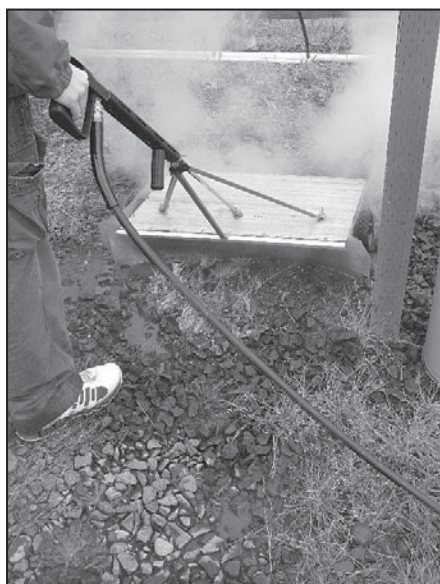
Figure 7. Testing a wet steamer to control weed growth.
