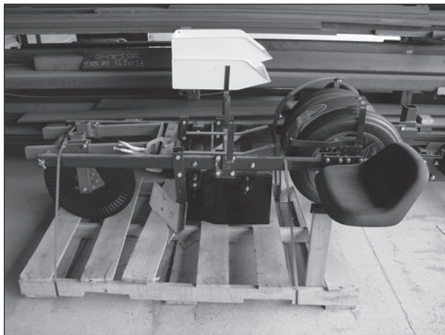
Figure 2. ATV-pulled mechanical tree planter.
