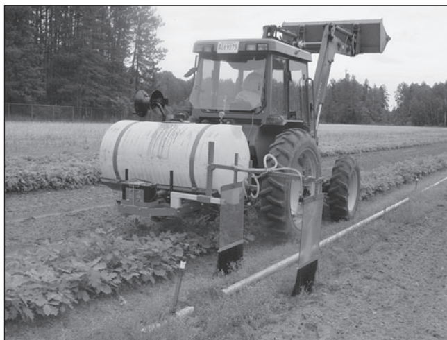
Figure 11. A sprayer shield assembly is shown mounted to a three-point hitch sprayer designed specifically for spraying around irrigation pipelines.
