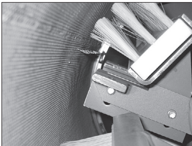
Figure 5. Brush-cleaning combs keep awns from clogging rotating brushes in a Westrup HA-400 (Huntsman, Incorporated, Twin Falls, ID).
