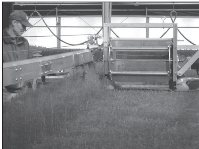
Figure 6. A top pruner designed for trimming container seedlings.
