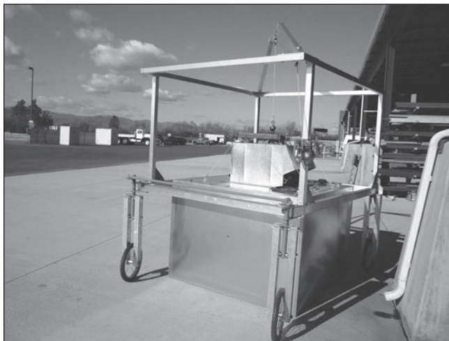
Figure 4. An in situ freeze chamber developed to simulate freeze events on bareroot seedlings.
