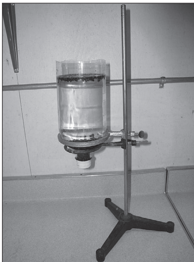
Figure 7. A large plastic soda bottle can be used to separate seeds in the Imbibe, Dry, Separate (IDS) procedure.
