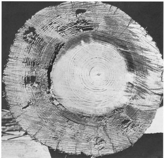
Figure 20.—Moderate decay (in-between pattern), hollows beginning to form.
