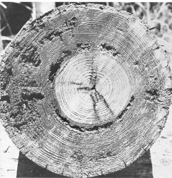
Figure 21.—Advanced decay (in-between pattern), only the central heartwood is sound. (The highest electrical resistance measurements will be in the central heartwood).
