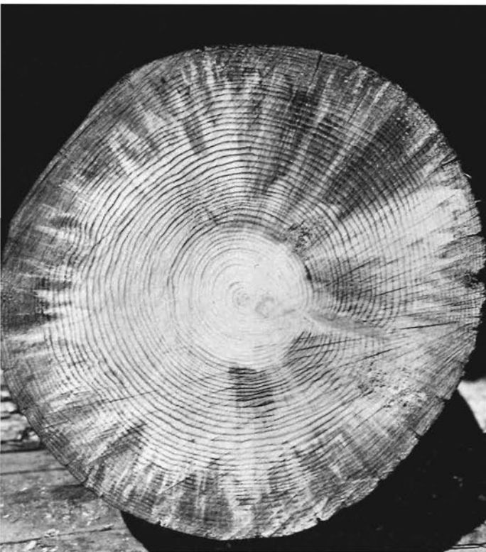
Figure 36.—Bluestain in a pole. The stain pattern can occur rapidly on the cut ends of freshly cut tree trunks. The stain may block the penetration of preservatives.
