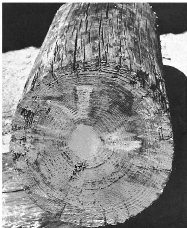
Figure 13.—Shell rot (external decay).
