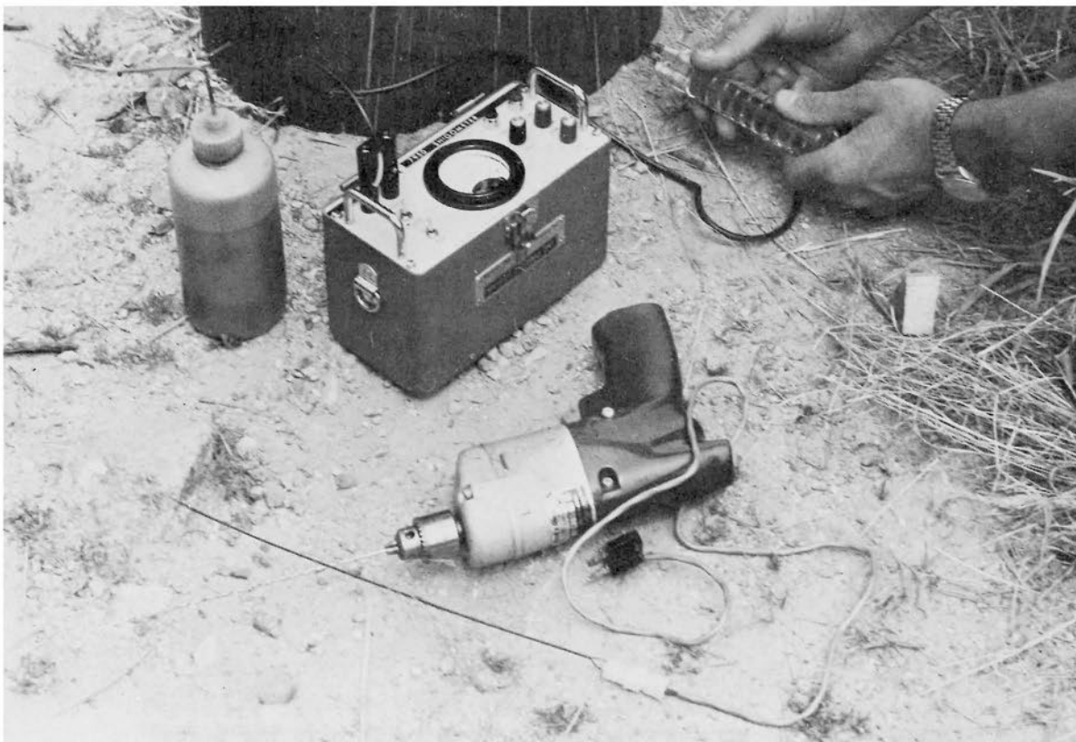
Figure 5F.—Probe around the base of the pole with the needle probes. When the probes go easily into the wood decay is suspect. Probe only with the needles aligned vertically as shown. Probe into checks also.
