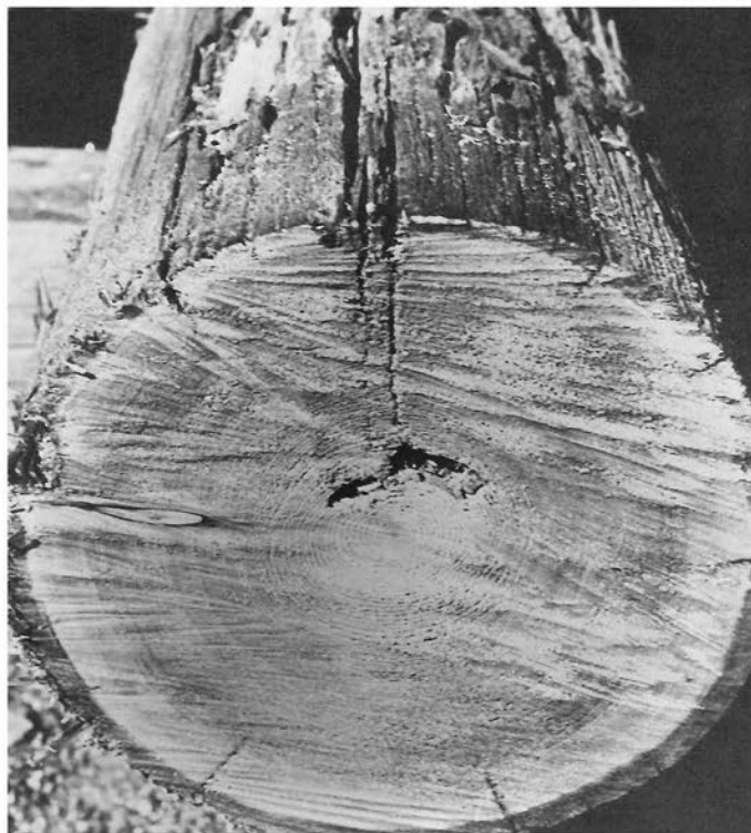
Figure 26.—Deep checks as entrance holes for ants that were in the central hollow.
