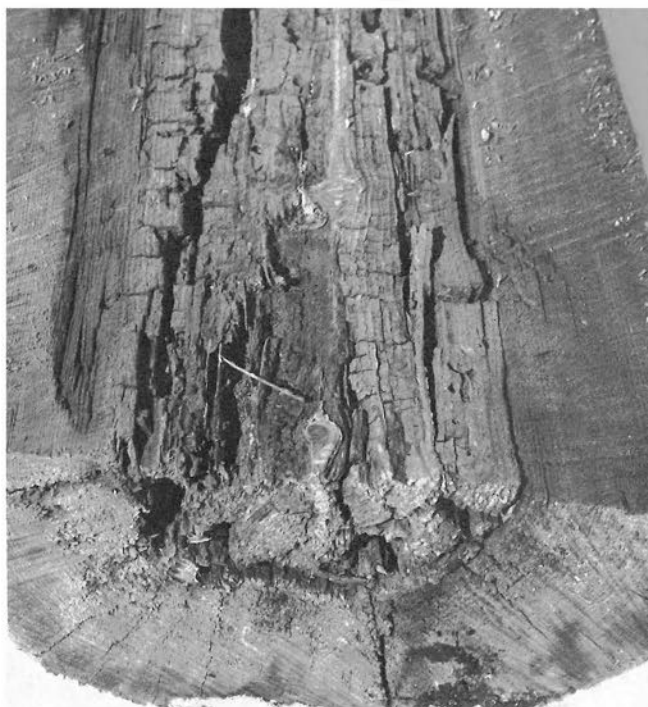
Figure 12B.—Radial section of complete decay.
