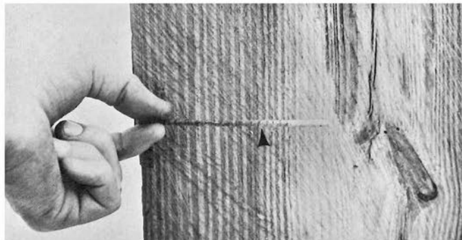
Figure 33.— Core from an increment borer at the exact position as shown. The wood at the inner portion of the core would appear sound to the eye. The Shigometer would indicate that the wood was beginning to decay. The core was taken only a few inches beyond the margin of the obvious column of decay. With the Shigometer it is not necessary to drill exactly into the column of obvious decay in order to detect it.
