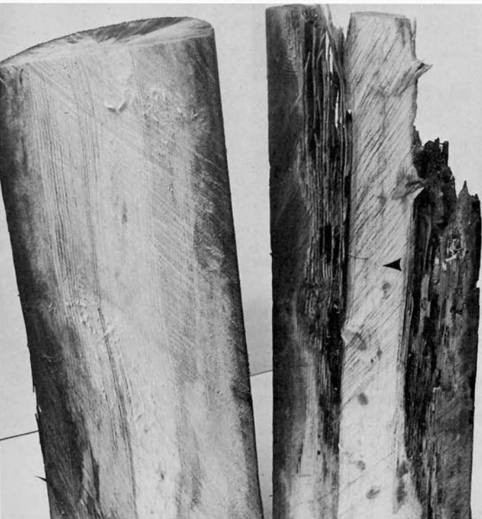
Figure 38.—The arrow shows the groundline. Note the sound heartwood core and the abrupt end to the decay. The section on the left was below the other, deep in the ground.
