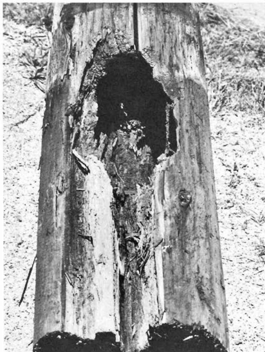
Figure 24.—Large holes are obvious signs of internal decay and hollows.
