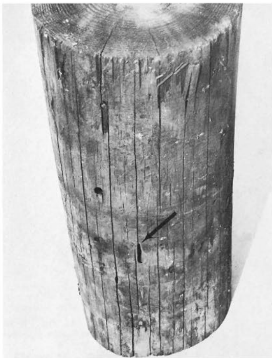
Figure 27.—Holes with smooth margins (arrow) often indicate entrance ports for ants.
