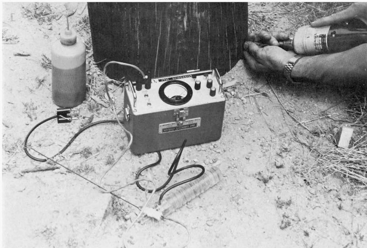
Figure 5D.—Cup hand around drill bit and guide it to the proper position and angle. If drilling is difficult and the bit gets hot, let the hole cool for a few minutes before inserting the twisted-wire probe.
