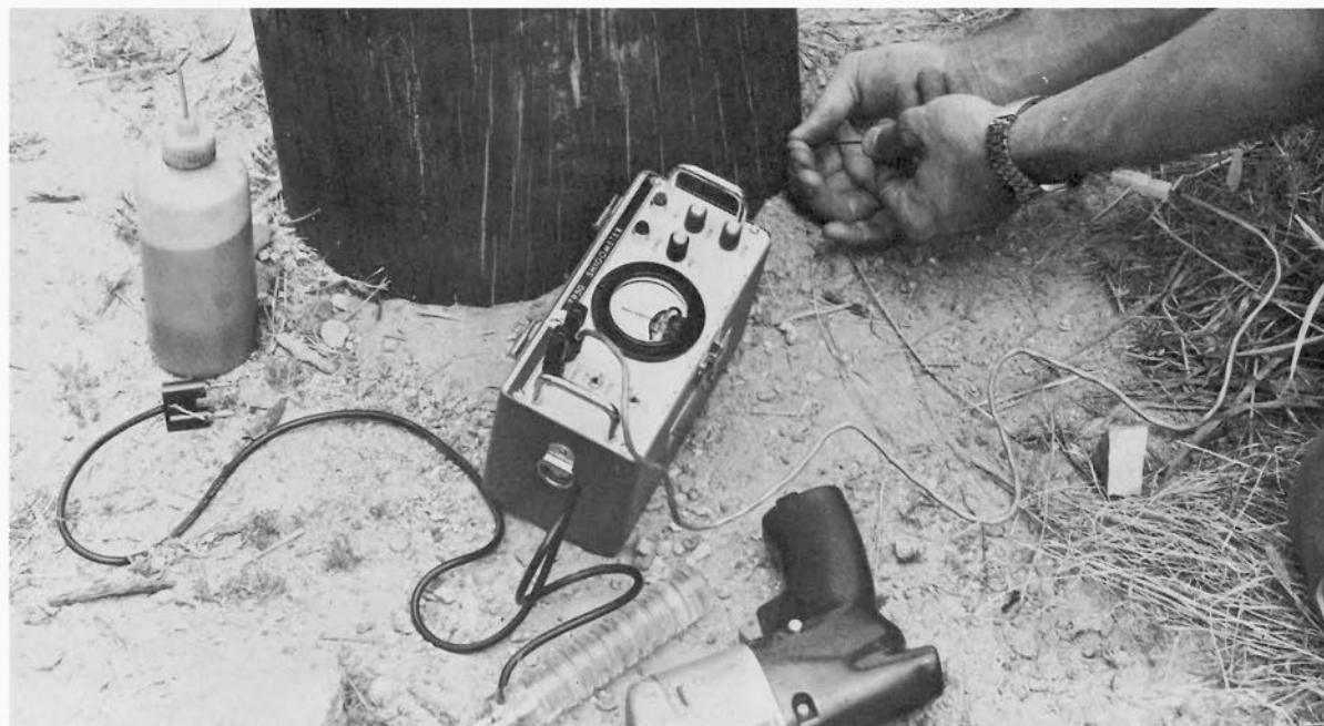
Figure 5E.—Insert twisted-wire probe slowly, and watch the dial on the meter as you momentarily release your fingers from the probe. Make certain that the probe is pushed in only a quarter of an inch at a time. Hold finger on probe close to the pole; this will prevent the probe from bending.
