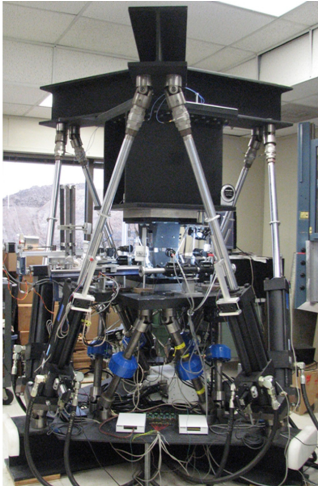
Fig. 1 NRL66.3: Most recent 6-DoF mechatronically automated system for the multi-axial testing of materials
