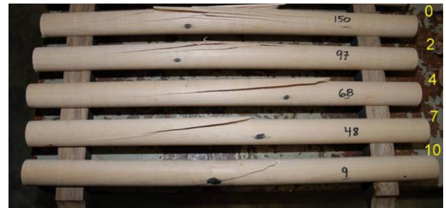
Figure 7: Example of the changing failure mode with increasing SoG. The SoG of the test specimens increase from top to bottom. The target angle category for each dowel is shown in yellow.
