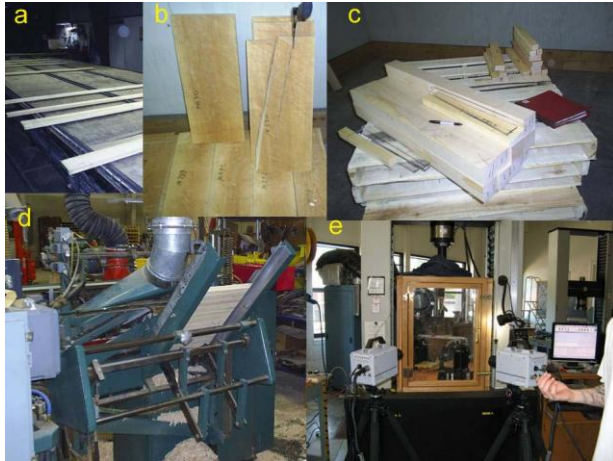
Figure 4: Summary photo of dowel preparation: a) board selection, b) section splitting, c) marking section with template, d) dowel manufacture, e) universal test setup
