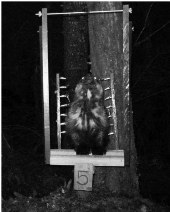
Figure 4. Photograph of a wolverine taken with a motion-detection camera at a camera and hair-snap station in Southeast Alaska, USA, in 2010 showing the ultra high molecular weight (UHMW) plastic uprights and steel crossbar and 2 UHMW plastic hair-snap posts with 7 base clips and trigger clips per post.
