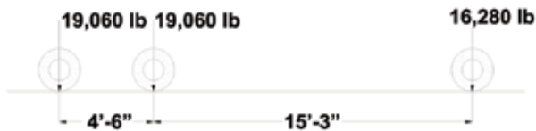
Figure F8. Truck Configuration and Axle Loads
