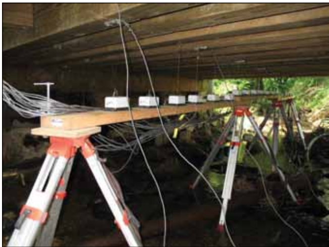
Figure J6. Deflection instrumentation.
