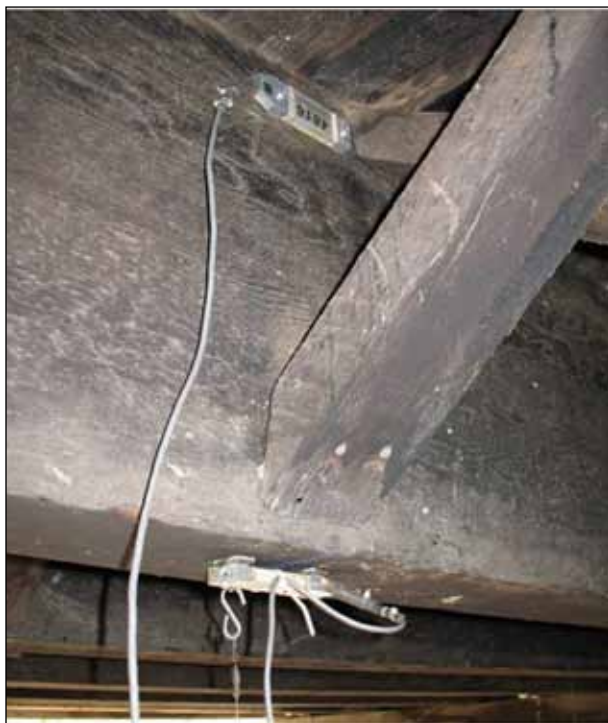
Figure N7. Strain transducers.
