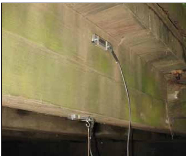
Figure G7. Strain transducers.
