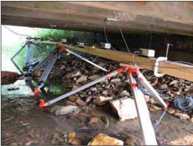
Figure E6. Deflection instrumentation.
