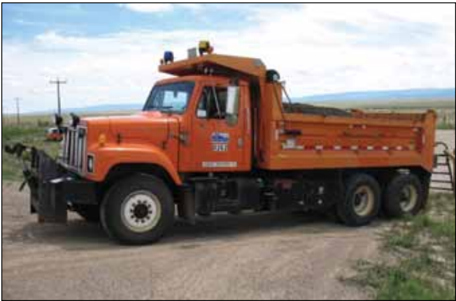
Figure L9. Tandem-axle load truck.
