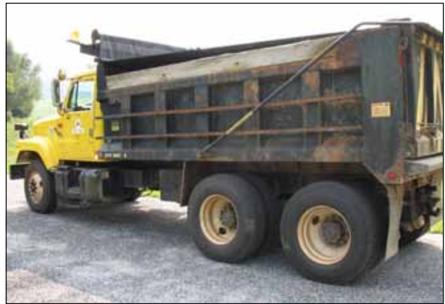
Figure E9. Tandem-axle load truck.
