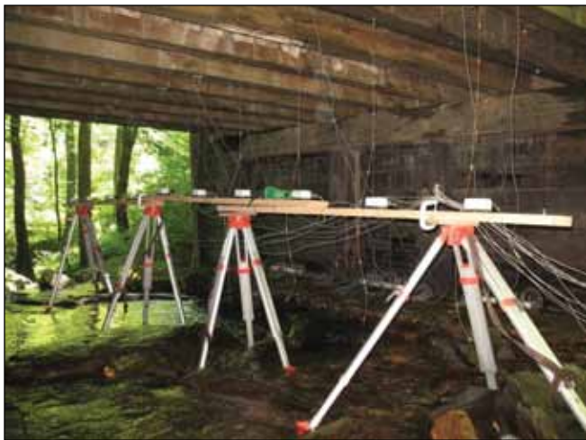
Figure F6. Typical deflection instrumentation.
