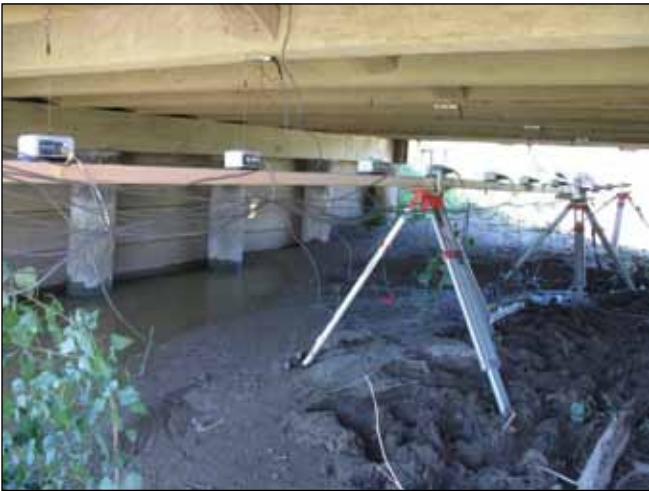
Figure M6. Deflection instrumentation.
