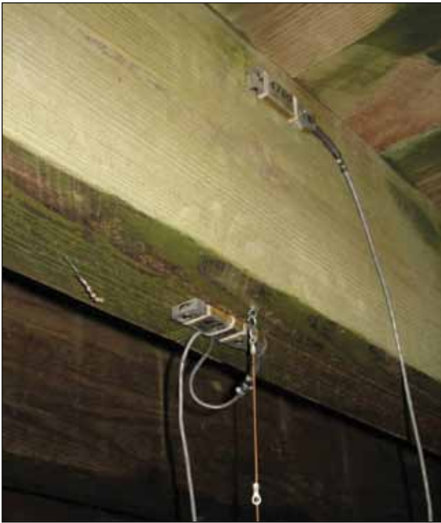
Figure 6. Typical strain transducer placement.
