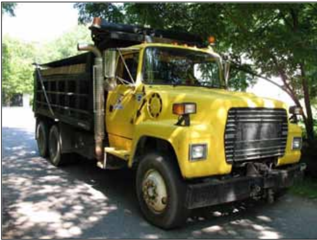
Figure C9. Tandem-axle load truck.
