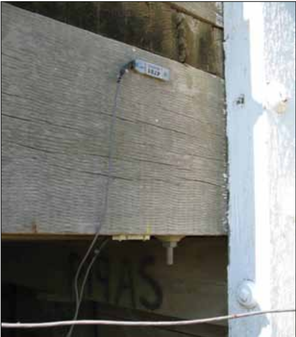
Figure M7. Strain transducers.
