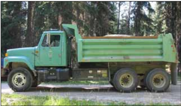
Figure P9. Tandem-axle load truck.
