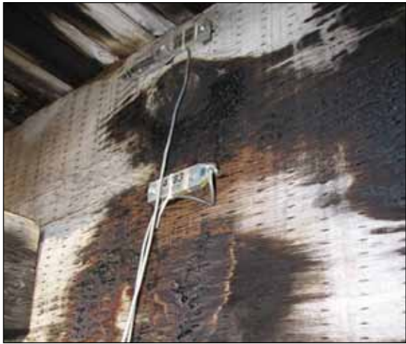
Figure P7. Strain transducers.
