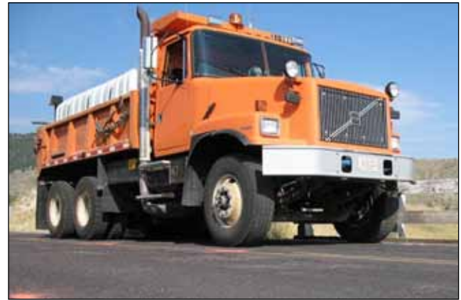
Figure O9. Tandem axle load truck.
