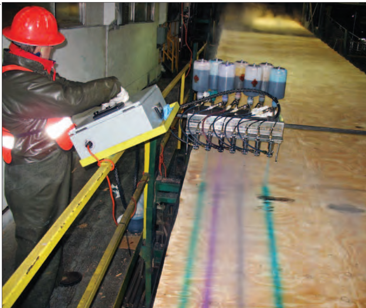
A technician marks veneer sheets to determine if wood-product properties can be predicted from acoustically tested tree properties.
