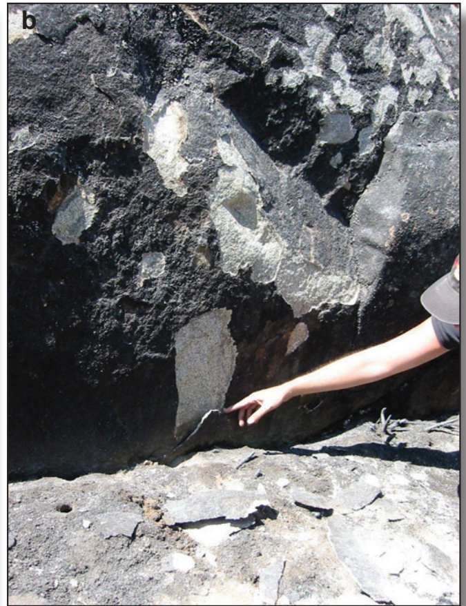
Figure 4-9 —(a) Heavy brush (manzanita) growing at the base of this granite face resulted in severe localized spalling. (b) Spalled fragments remaining attached to this granite face were easily removed by the touch of a finger.
