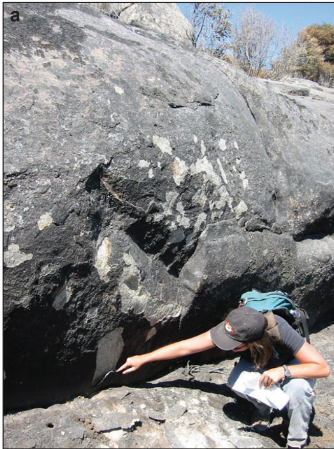
Figure 4-9 —(a) Heavy brush (manzanita) growing at the base of this granite face resulted in severe localized spalling. (b) Spalled fragments remaining attached to this granite face were easily removed by the touch of a finger.
