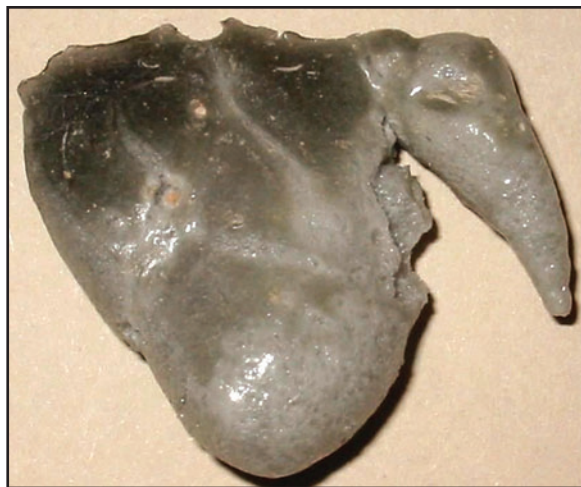
Figure 4-3 —Bloated and melted obsidian, oven heated to 800 °C (1472 °F) (sample courtesy of Anastasia Steffen).
