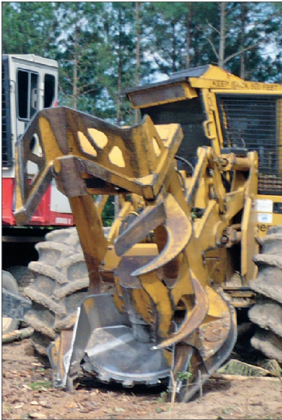
Improvements in harvesting machines cut most trees near ground level and increases utilization. (photos by Tony Johnson, Southern Research Station)
