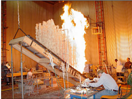
Lab scientists Mark Finney and Bret Butler conduct an experimental burn in the Fire Sciences Laboratory large combustion chamber.
