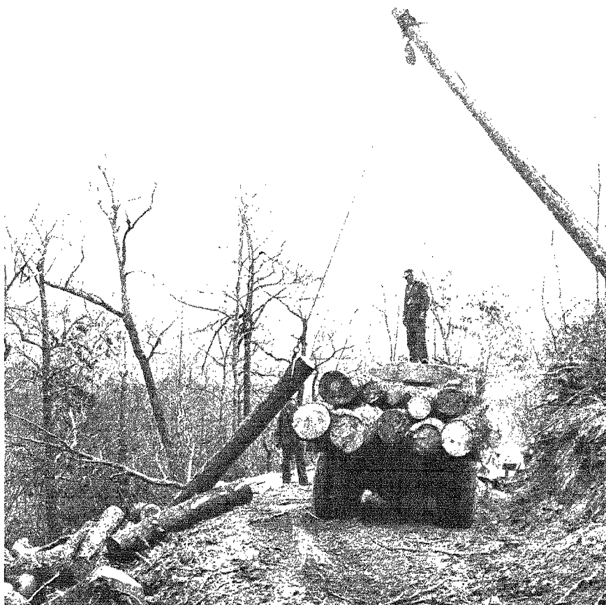
Figure 19.—A-frame yarding logs on steep mountains near Franklin, North Carolina, 1952. Both A-frame sites and skid paths were fully revegetated and could not be traced by 1960.
