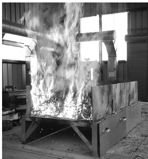
Fig. 1. Fuel bed constructed of live foliage and branches of chamise with 2.0 m long, 1.0 m wide, and 0.4 m depth. The fire illustrates the initial ignition.
