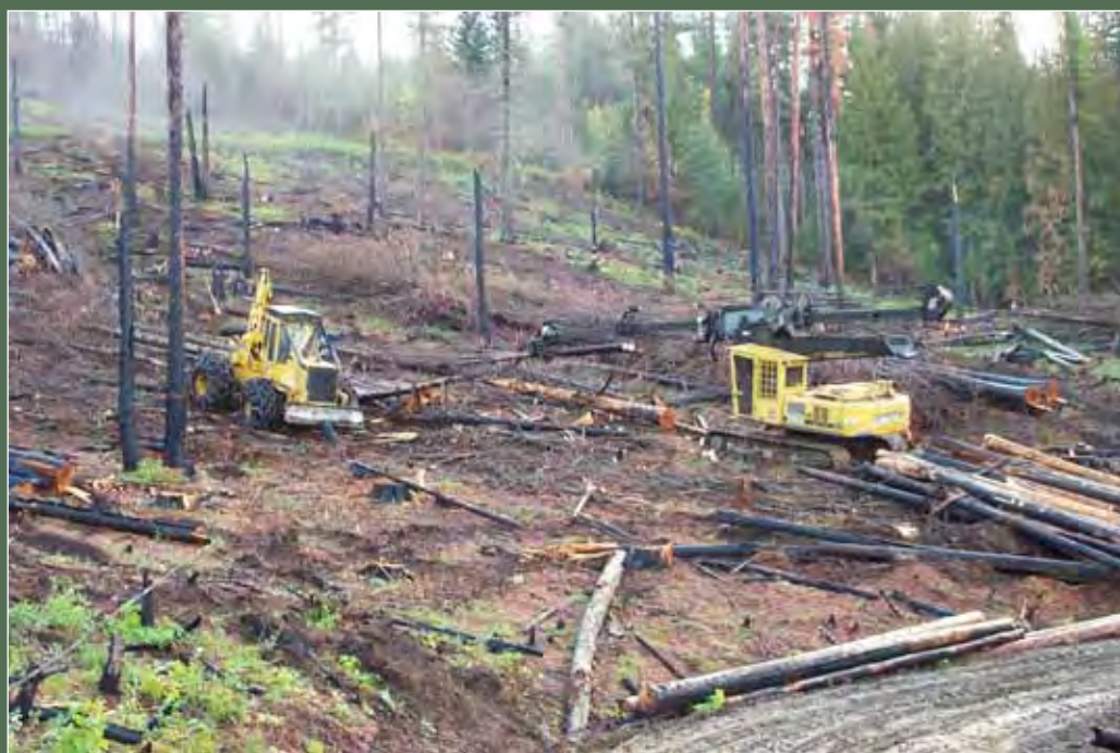
Skidder and delimber operating on a fuel management research project in the Priest River Experimental Forest in Idaho.
