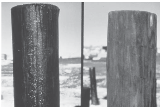
Figure 11.2 Traditional (left) and BMP creosote piling.
