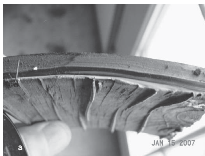
Figure 11.11 (a) Breach of the TIP HDPE piling wrap with adhered surficial layers of ACZA treated wood and (b) breach of the untreated piling with no adherence of the underlying wood fibers.
