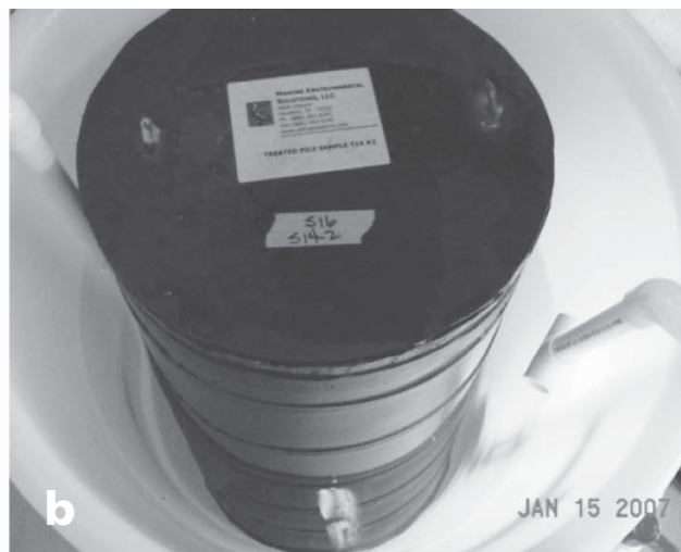
Figure 11.9 ACZA-treated piling wrapped with (a) Port of Los Angeles inner petrolatum saturated tape and 30 mil outer wrap of polyvinylchloride (PVC) or (b) TIP-HDPE.
