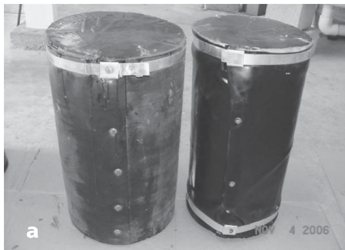
Figure 11.9 ACZA-treated piling wrapped with (a) Port of Los Angeles inner petrolatum saturated tape and 30 mil outer wrap of polyvinylchloride (PVC) or (b) TIP-HDPE.
