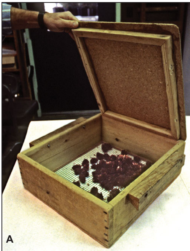
Figure 2.9 —Wooden frame boxes with screened bottoms (A) can be used to separate seeds from other debris. Depending on the type of dry fruits and seed size, several boxes with different sized mesh may be needed. With gentle shaking over a series of screens, pure seeds can eventually be obtained (B).
