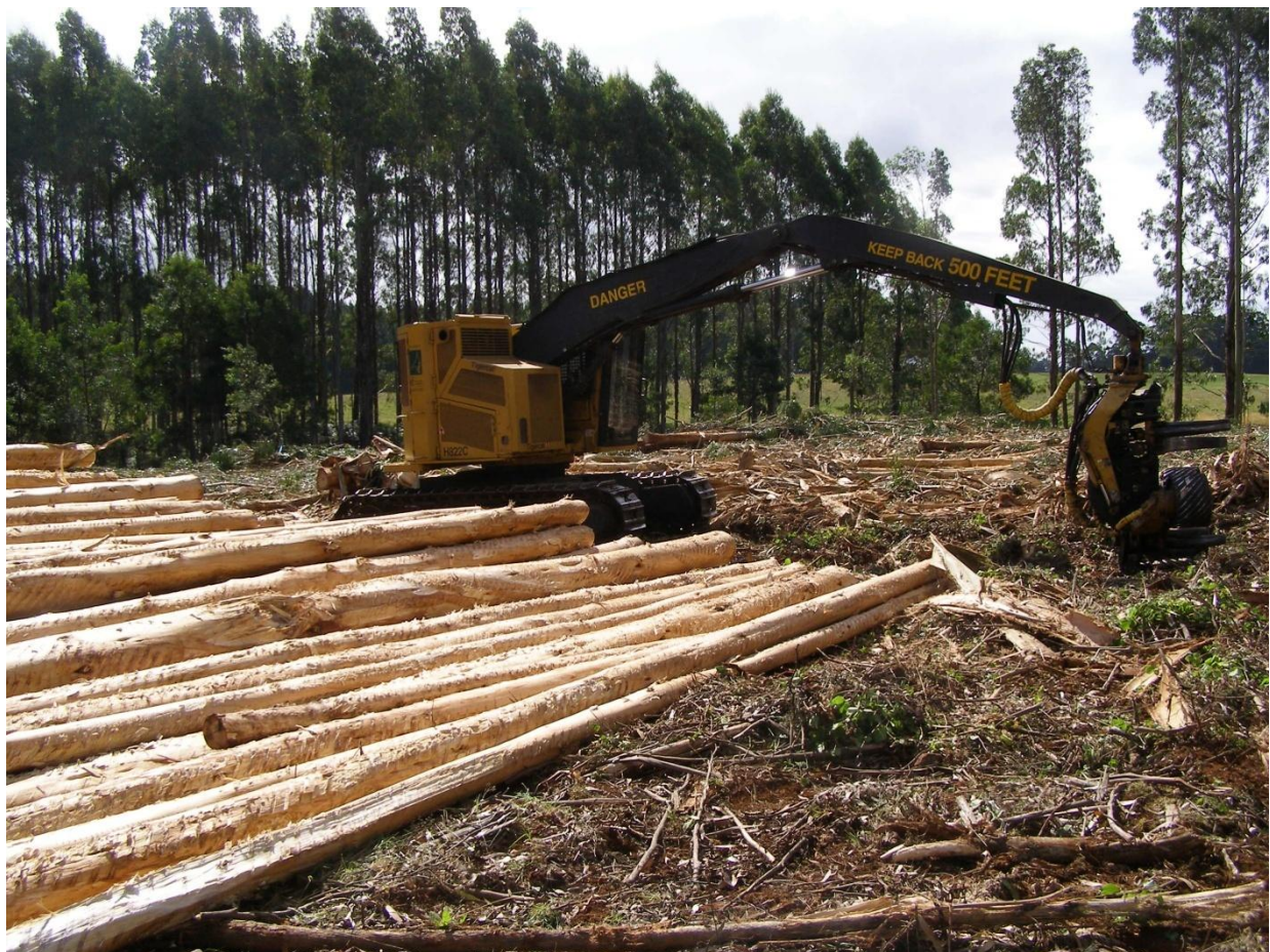
Figure 20. Tigercat tracked harvester stacking delimbed and debarked Eucalyptus nitens stems during an SMZ harvesting study that utilized Best Management Practices. Note the slash coverage remaining in the harvested area. Trees were harvested to the edge of the stream, which flows between the harvested and un-harvested area in this photo. (Photo by Daniel G. Neary)
