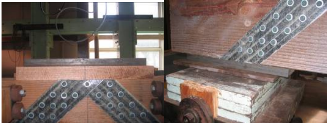
Figure 56: Steel and wood plates to remedy stress concentrations at both (a) the load head and (b) supports.
