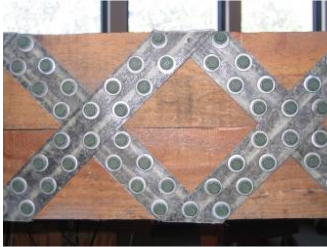
Figure 38: FRP X-braced specimen finished product. Each beam was 4” deep and the system was a total of 8” deep. Note a missing screw at the top where strips overlapped; in some cases the hole was too close to the edge of the beam and would cause splintering if drilled, or a knot in the wood prevented a screw from being placed.
