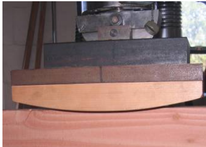
Figure 34: Detail of Width Series load head. The point of contact is made of hardwood mounted to a steel plate and then the load cell.
