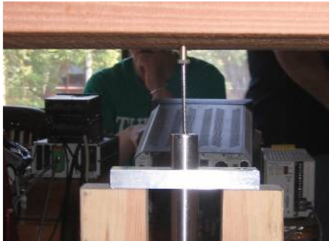
Figure 33: Quarter span LVDT held in place at the center of the beam thickness by a clamp and stand.
