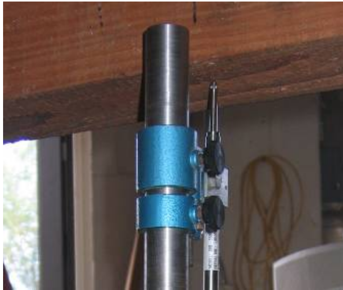
Figure 31: Mid span LVDT held in place at the center of the beam thickness by a clamp and stand.
