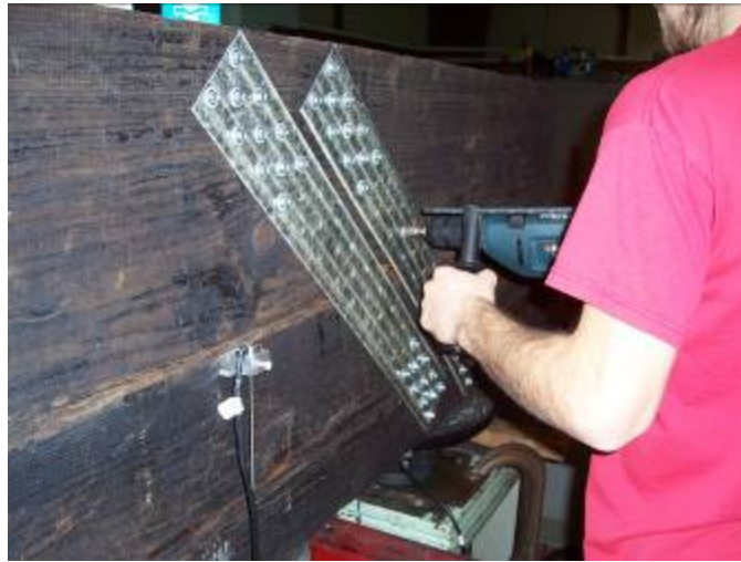
Figure 63: MF-FRP specimen fabrication. 12" x 12" stacked beams had 4" strips applied with lag screws directly in the test set up. Note that not all of the pre-drilled holes are being used.
