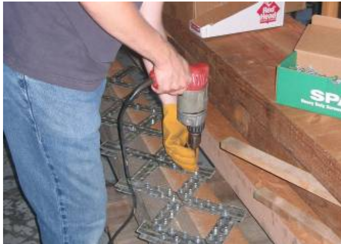
Figure 36: MF-FRP Specimen fabrication. 1.75" wide FRP strips were attached to timber specimens using Spax self tapping lag screws. This did not require any special training or equipment, and could be done easily by students using simple tools.
