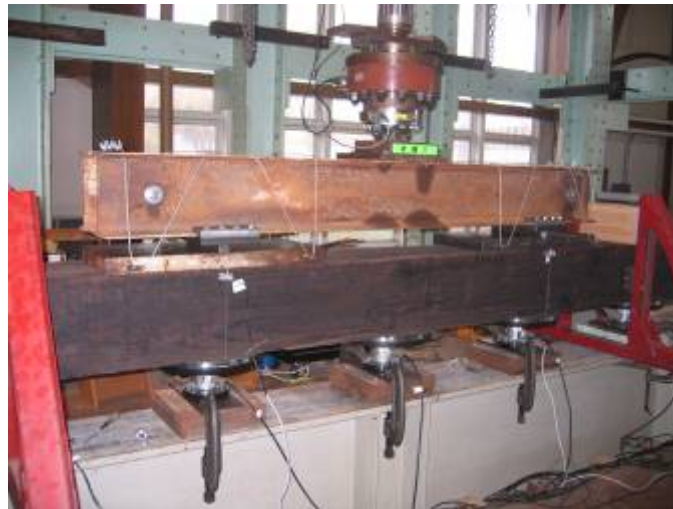
Figure 60: Phase 2 test setup, with the 3 center supports visible.
