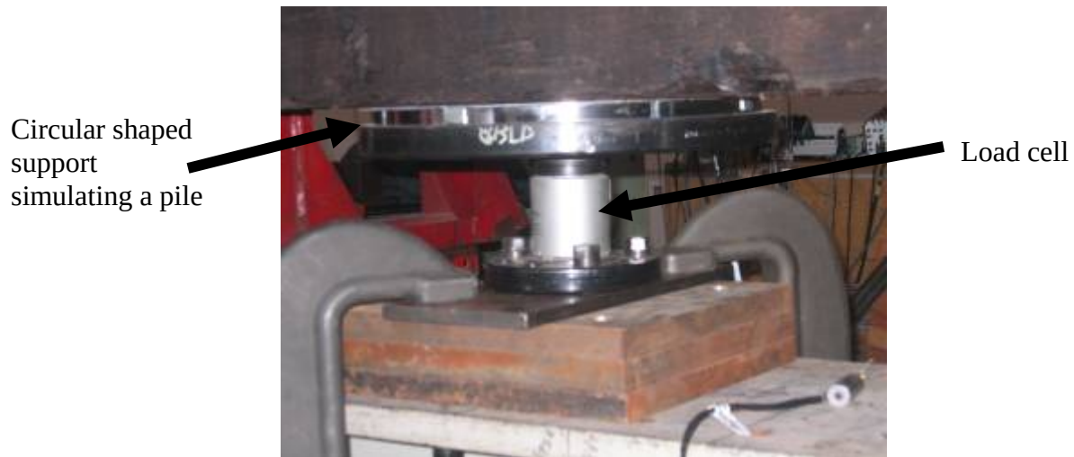
Figure 62: Detail of load cell at support.
