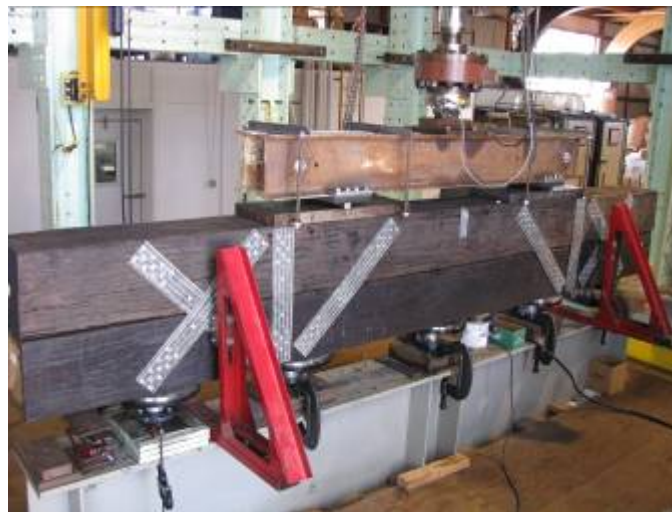
Figure 69: Combination of compression and tension strips.
