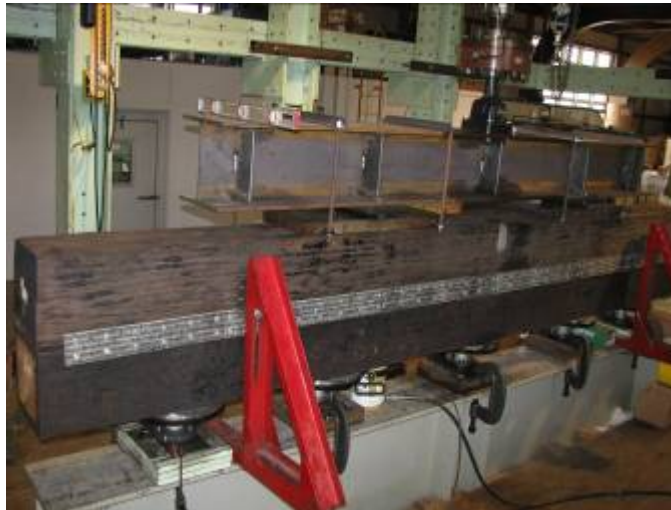
Figure 68: Horizontal strips at double cap interface.
