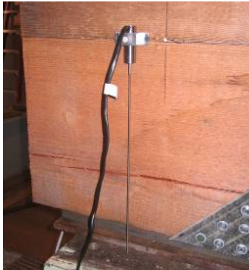
Figure 53: LVDT measuring transverse compression in wood.
