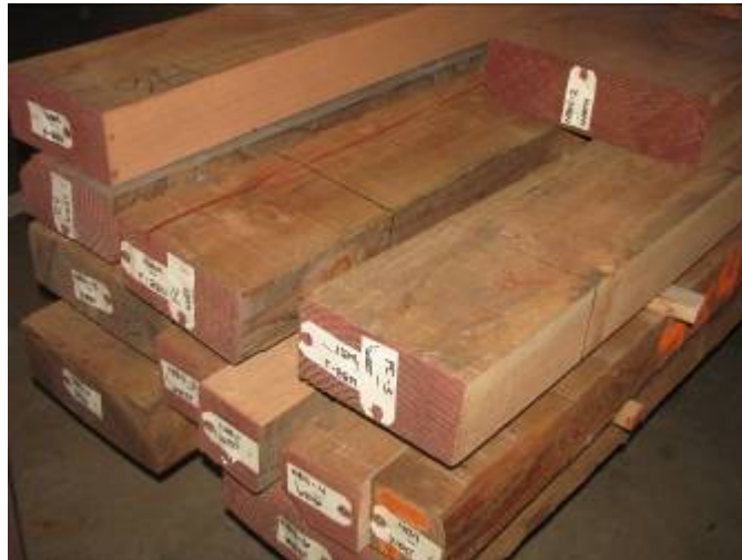
Figure 22: Rough sawn Douglas Fir specimens out of storage at the Forest Products Lab in Madison, WI.
