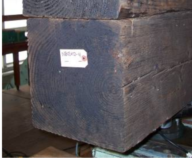
Figure 23: Full sized 12" x 12" creosote treated specimen.
