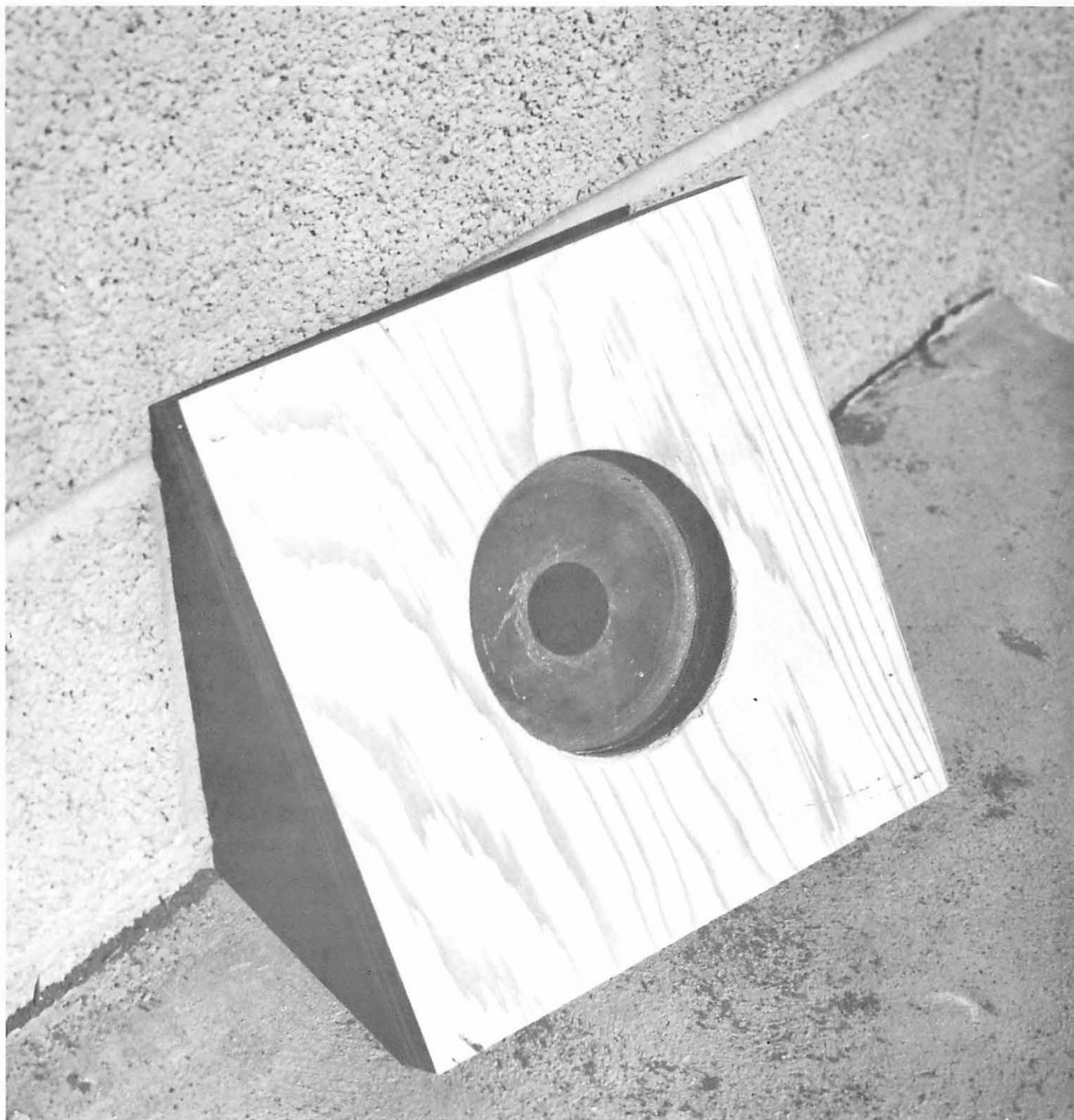
Figure 7. --Lens board and back board glued together and ready for mounting in the box. View is from the underside. The shutter is attached to the upper side and the Graflok back to the underside.
