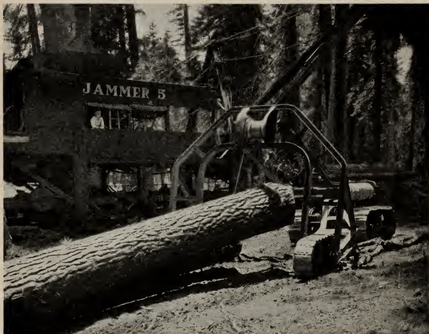
Fig. 11.—Fair-lead wheel yarding. Note the drum mounted on the rear of the tractor, for hauling in the logs. This big wheel is equipped with Athey truss wheels. It is also equipped with the same type of wheel as shown in figure 5. (Photo by courtesy of the Caterpillar Tractor Co.)
