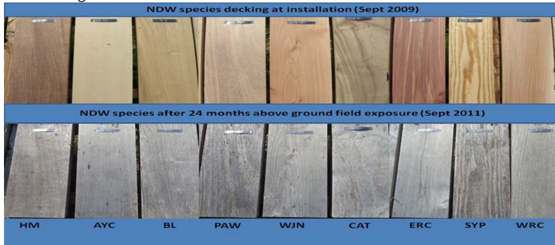
Figure 3: Composite image showing NDW decking specimens at installation (top) compared to NDW specimens after 24 months above ground field exposure (bottom). (HM=honey mesquite, AYC=alaska yellow cedar, BL=black locust, PAW=paulownia, WJN=west coast juniper, CAT=southern catalpa, ERC=eastern red cedar, SYP=southern yellow pine (control), and WRC= western red cedar.)
