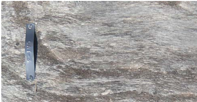
Figure 5: Cross checking of juvenile wood in Southern Catalpa after 12 months of weathering in WI.
