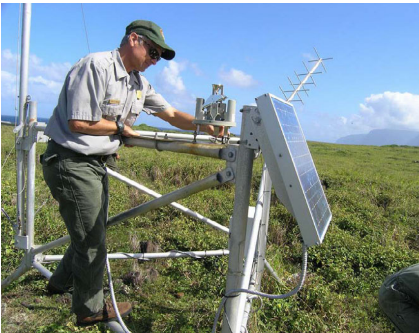
This Remote Automated Weather Station (RAWS) at Kalaupapa National Historical Park can be used to measure temperature as well as other climactic factors; NPS photo.
