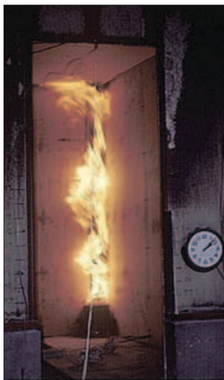
Figure 2. 100-kW flame at start of test.
