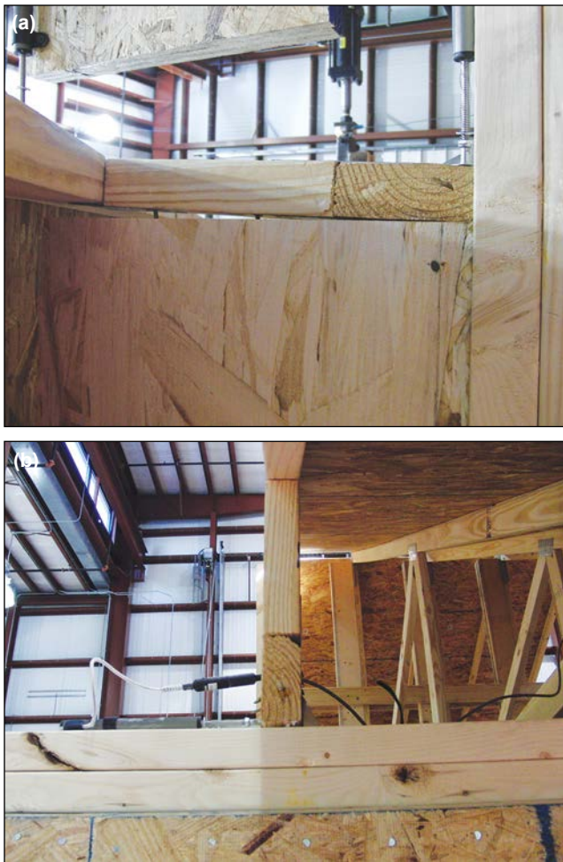
Figure 19. Comparison of truss heel rotation (Specimen F): (a) Truss 1, (b) Truss 5.
