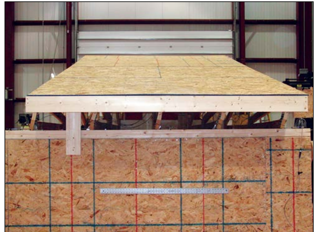
Figure 16. Specimen C heel rotation at failure.
