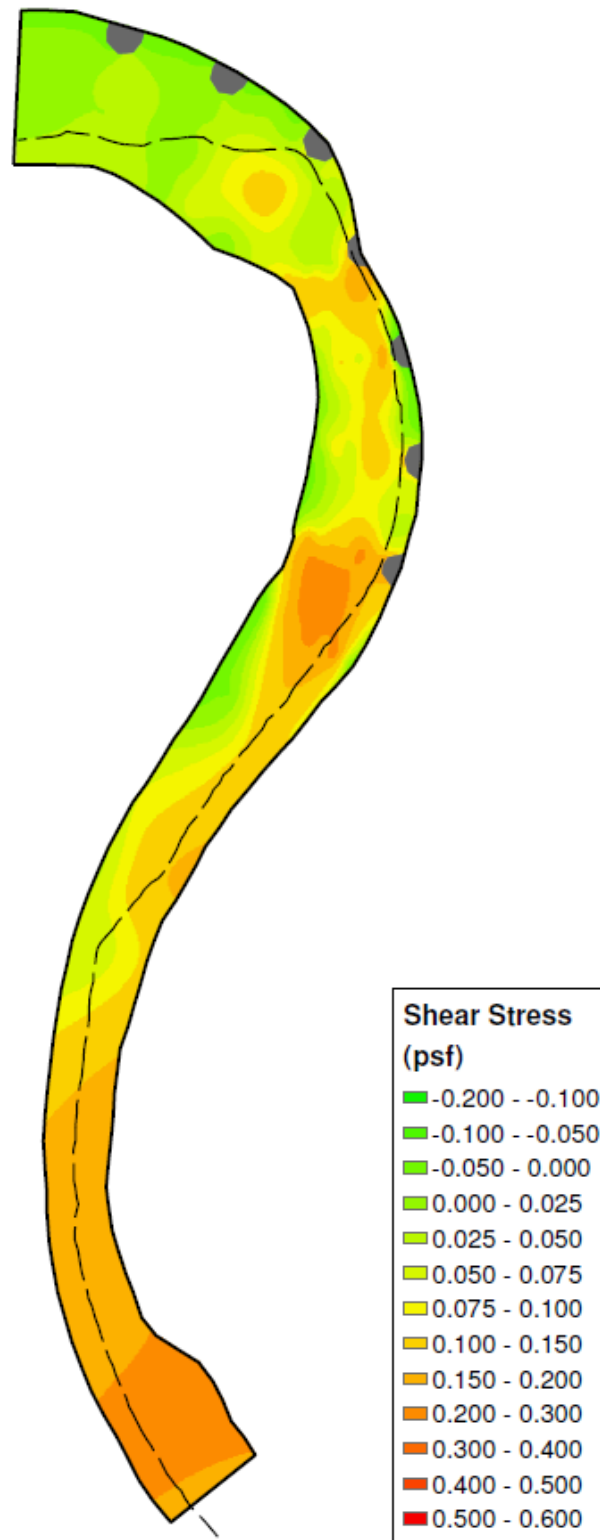
Figure D.4: NW04 Boundary Shear Stress Plot
