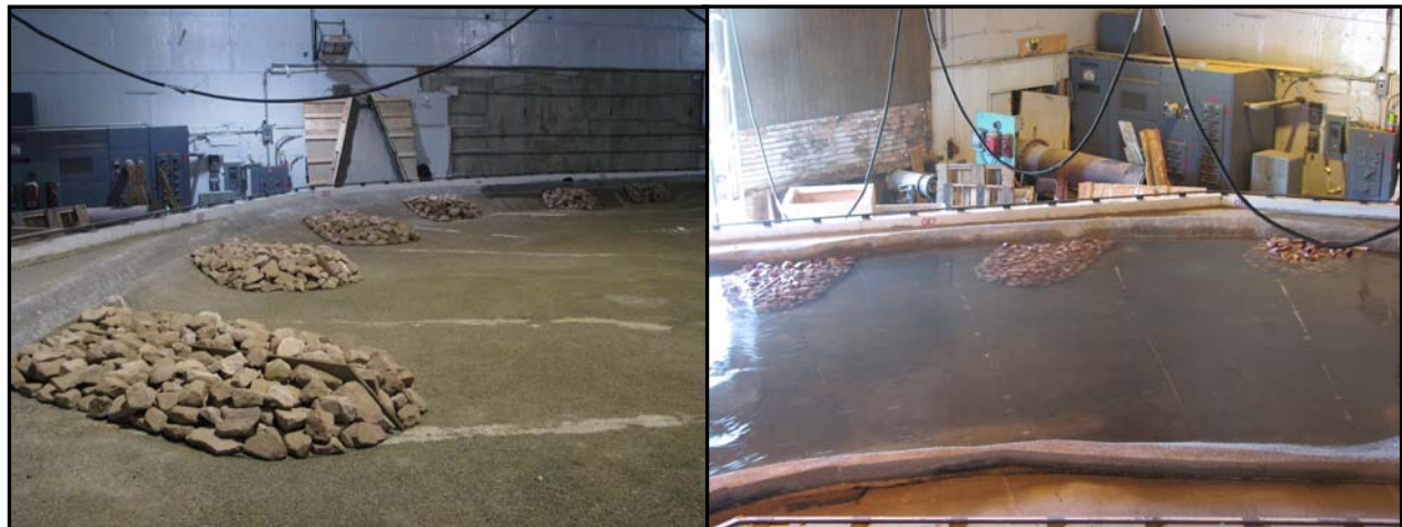
(a) installed spur dikes
