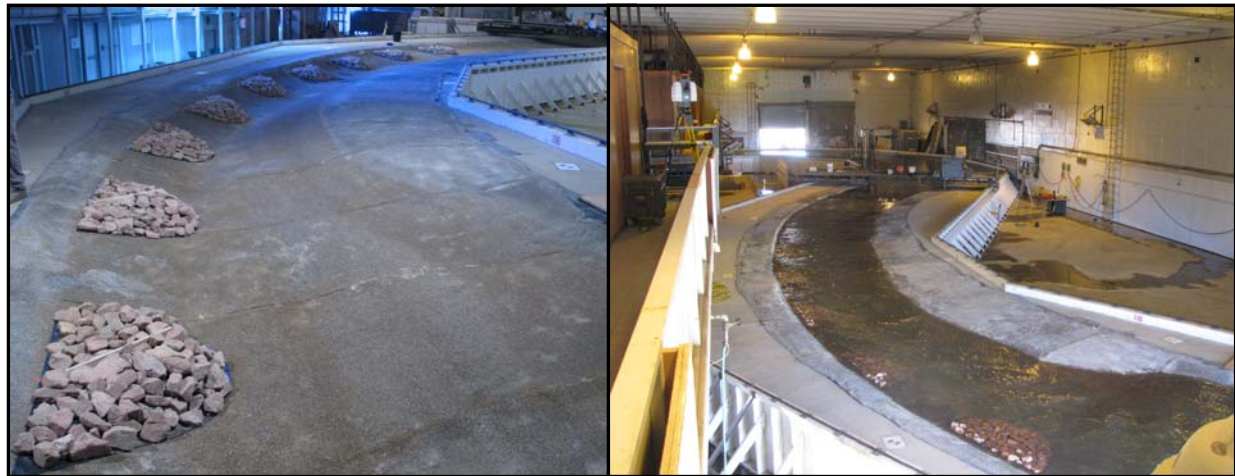
(a) installed spur dikes
