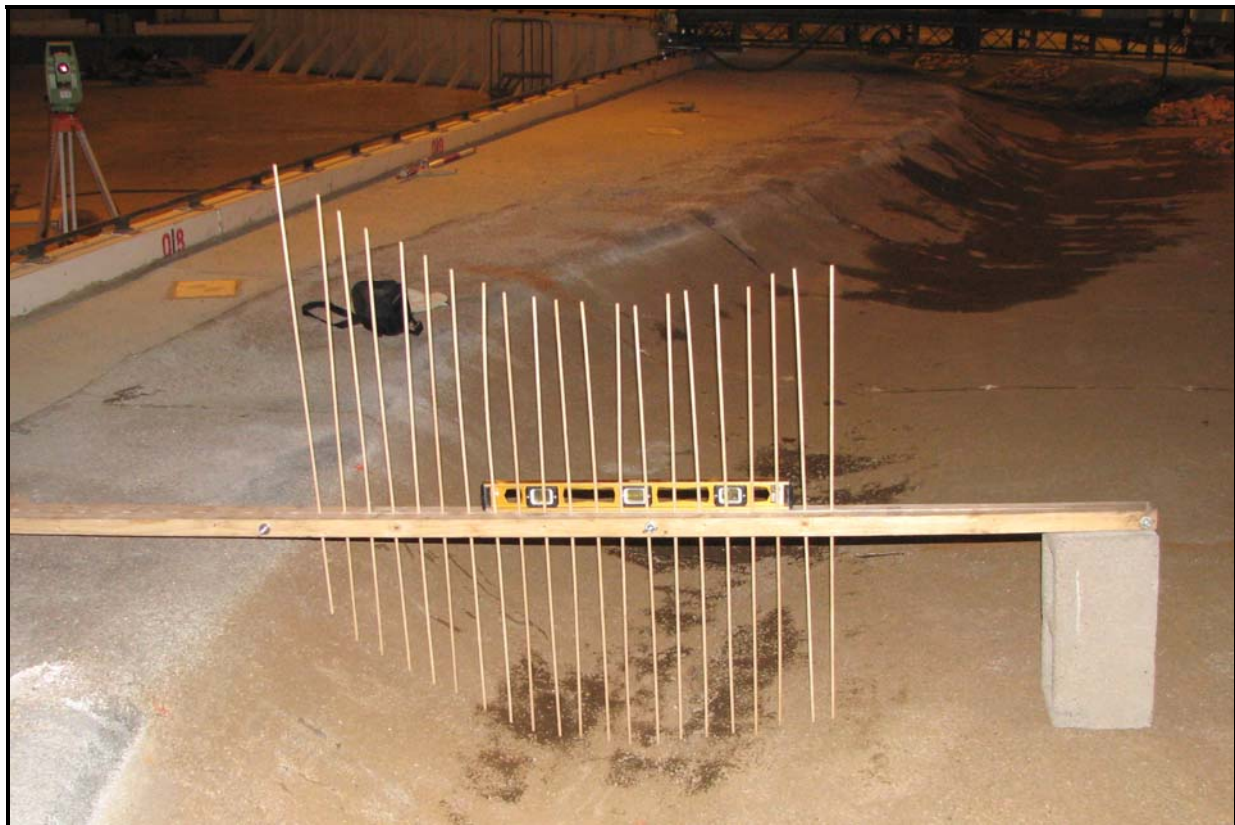
Figure 2.12: Dowel Bed-mapping Procedure
