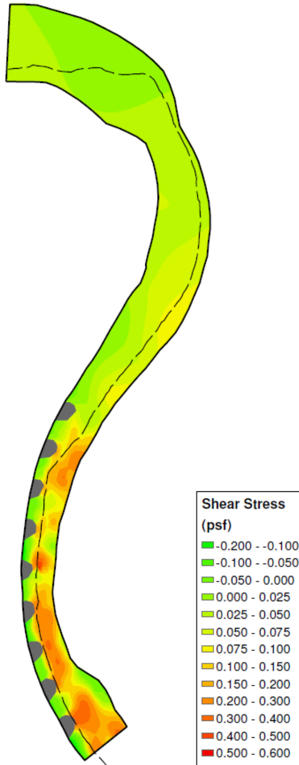
Figure D.3: NW03 Boundary Shear Stress Plot
