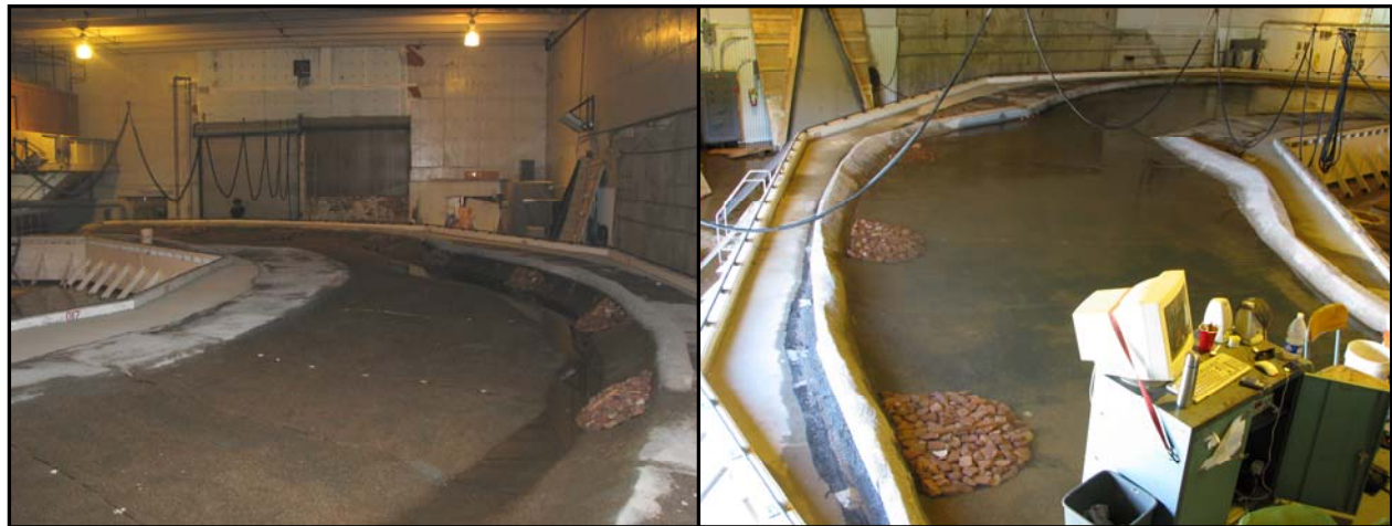
(a) installed spur dikes
