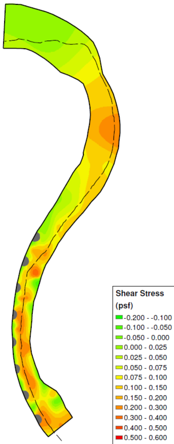
Figure D.1: NW01 Boundary Shear Stress Plot
