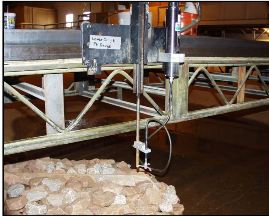
Figure 4.5: ADV Mounted on Point Gage and Data-acquisition Cart (Darrow 2004)
