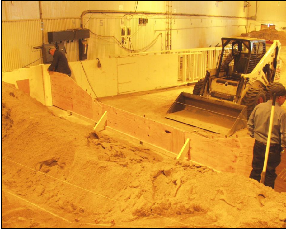
Figure A.6: Skeleton and Filling Material of the Main Channel
