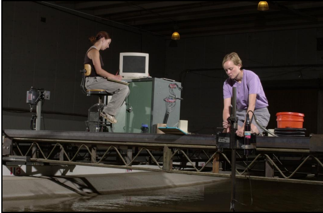
Figure A.17: Installation of the ADV in the Data-collection Cart
