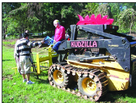
Figure 11. Kudzilla – kudzu root raking machine. Kudzu Coalition, Spartanburg, S.C. Image by Randy G. Westbrooks, U.S. Geological Survey, Whiteville, North Carolina.
