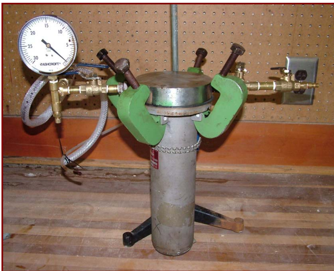
Fig. 1. Custom bench-scale vessel for high pressure treatment
