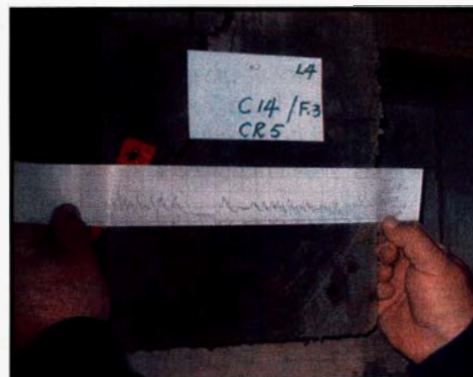
Figure 6 - Relative density plot from the resistance micro-drilling device held aligned to the drilling path.
