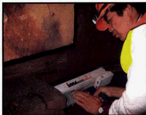
Figure 5 –Resistance micro-milling being performed at a foundation member.
