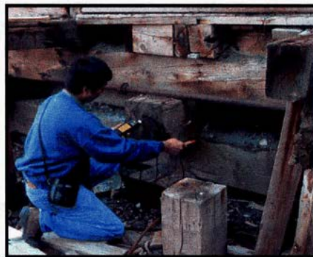
Figure 4 - Stress wave measurements being collected using a microsecond timer device.
