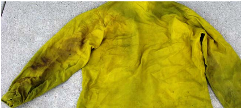
Dye sublimation and scorch on the back of the entire left arm and right elbow of shirt.
