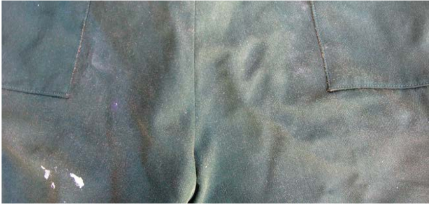
Dye sublimation (orange color) of the fabric fuzz and edges of rear pockets.
