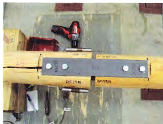
Figure 8: Typical Example of Douglas fir Type C bolt and plate connection failure
