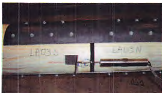
Figure 6: The ductile yielding of Type A thin plates and bending of structural screws accounted for the ductile nature of the structural screw connection system
