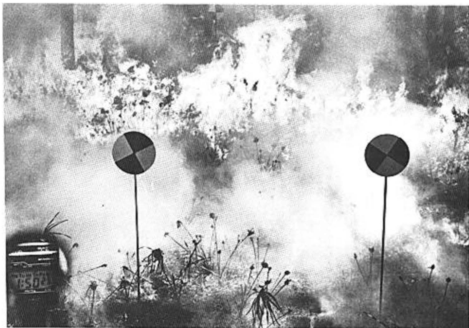
FIGURE 5. Head fire in the palmetto-gallberry fuel type with an average flame length of 1.20 m and a predicted source strength of 330,000 \mu\text{g m}^{-1} \text{s}^{-1} .
