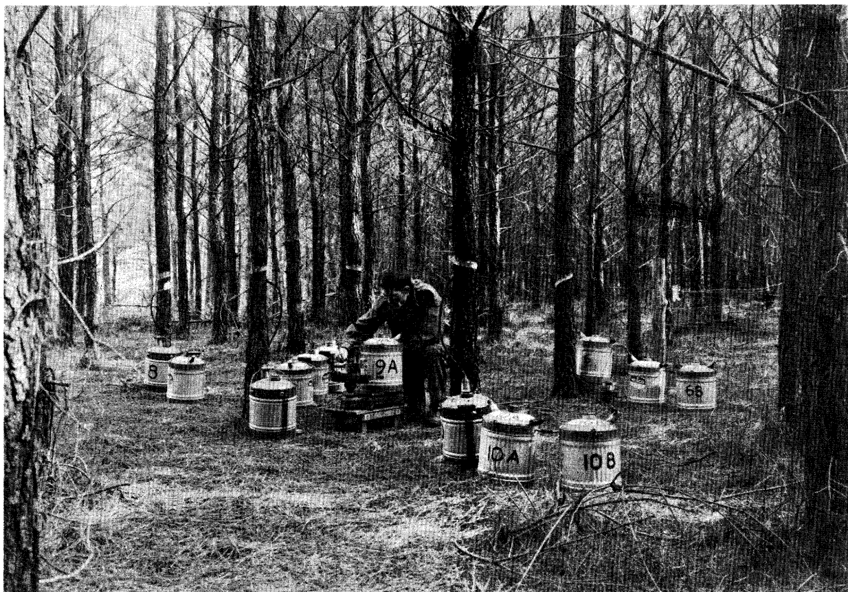
Figure 3.--Weighing the collection cans to determine amount of stemflow.
