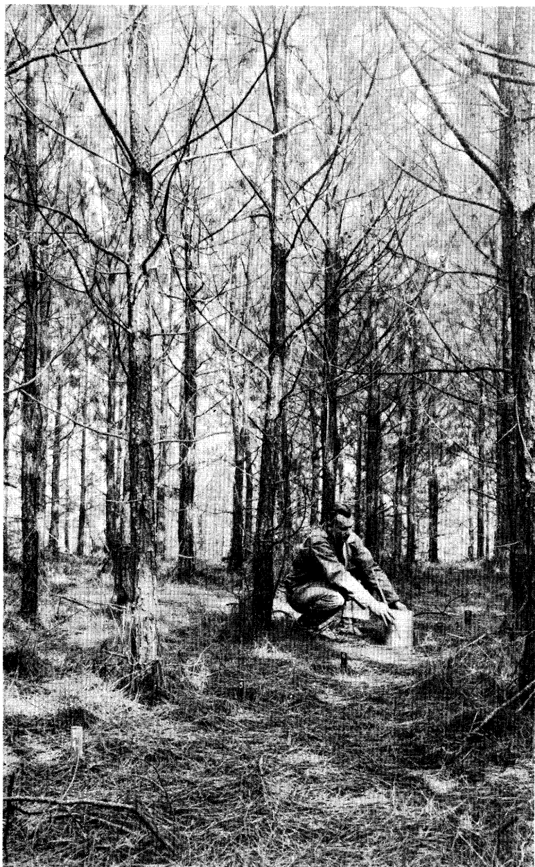
Figure 2.--Measurement of through-fall. Numbered stakes mark sampling positions. The undercanopy rain gages are set directly upon the ground. Note the upthrust branches of the young loblolly, believed to cause the high proportion of stemflow.
