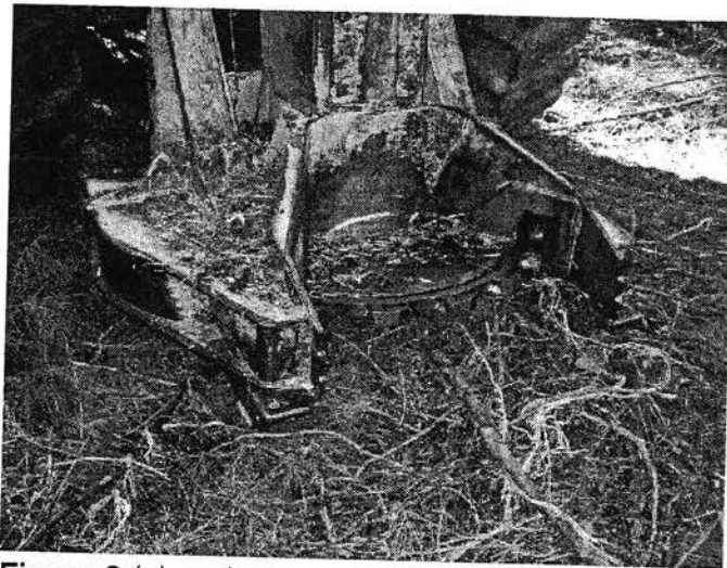
Figure 3 (above). Example of a cutting head from a feller-buncher.
