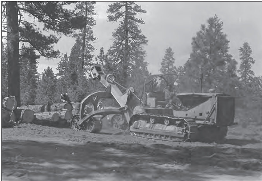
Figure 27—Early tractor with cleated tracks hauling logs. The use of tractors dramatically improved the efficiency of logging operations.
