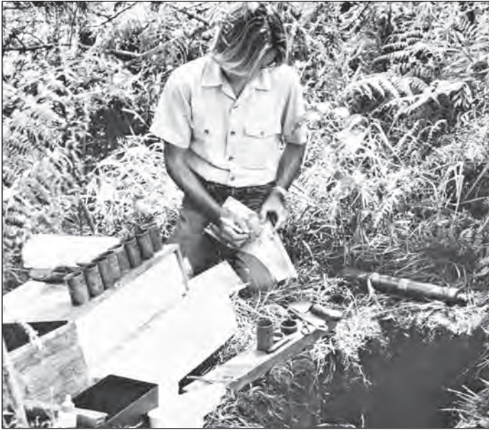
Figure 96—Sampling soils for hydrologic characteristics, 1977.
