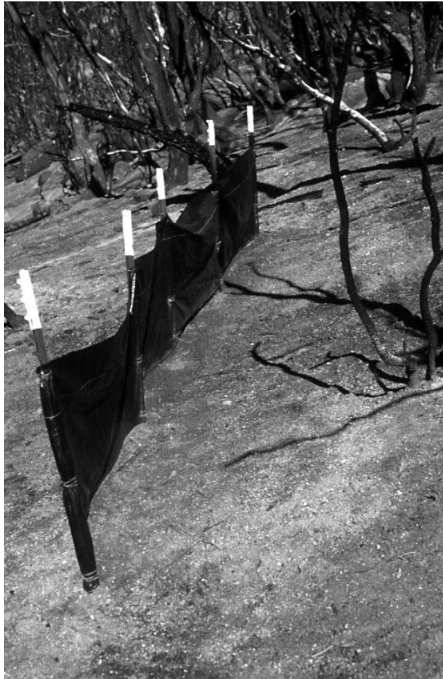
Figure 2. Photograph of a silt fence to measure surface erosion
