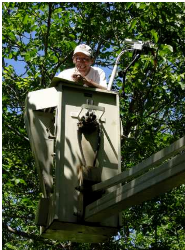
Figure 6: A photograph of leaf-level measurements being taken with a Li-Cor 6400 system. A cherry-picker allowed for vertical variations of sunlit- and shaded-leaf exchanges to be documented.
