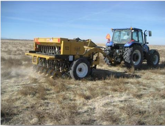
Figure 4. The Truax On-The-Go (OTG) Minimum-till Drill (left); broadcast seed box modification (right).
