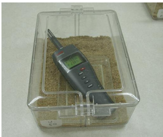
Figure 4. Equilibrium relative humidity (ERH) of seeds is measured with a hygrometer sealed in a test chamber with the seeds. Photo by Robert P Karrfalt, USDA Forest Service
