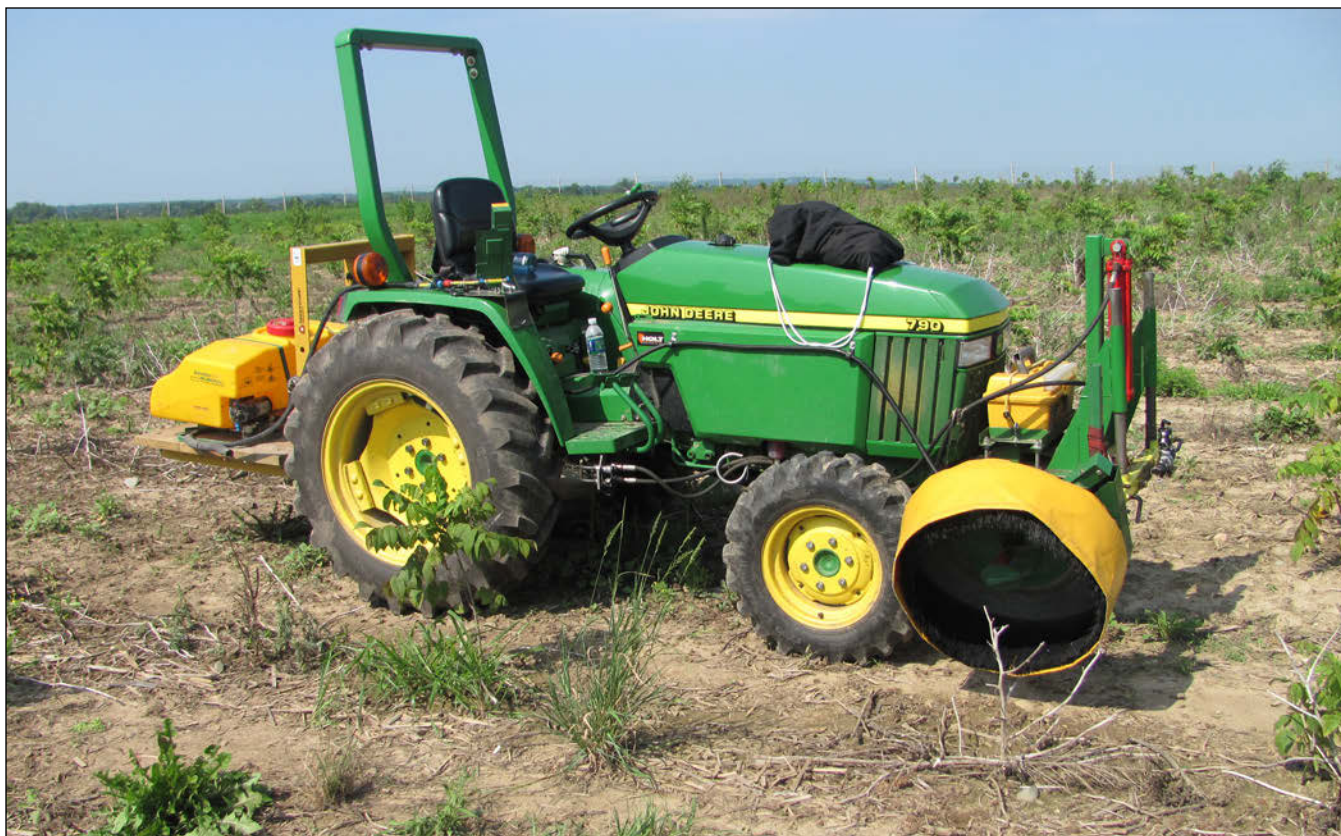
Figure 3.—Tractor-mounted control drop applicator with shield to control drift; this system is suitable for application of nonselective post-emergent herbicide. (Photo by J.W. Van Sambeek, U.S. Forest Service)
