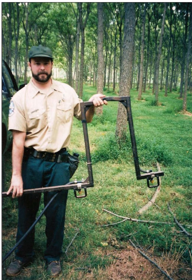
Figure 2.—Two nozzle tractor- or ATV-mounted boom for strip spraying young hardwood planting where height is adjusted so spray pattern of flat; fan nozzles are directed at base of tree seedlings and just barely overlap. (Photo by J.W. Van Sambeek, U.S. Forest Service)
