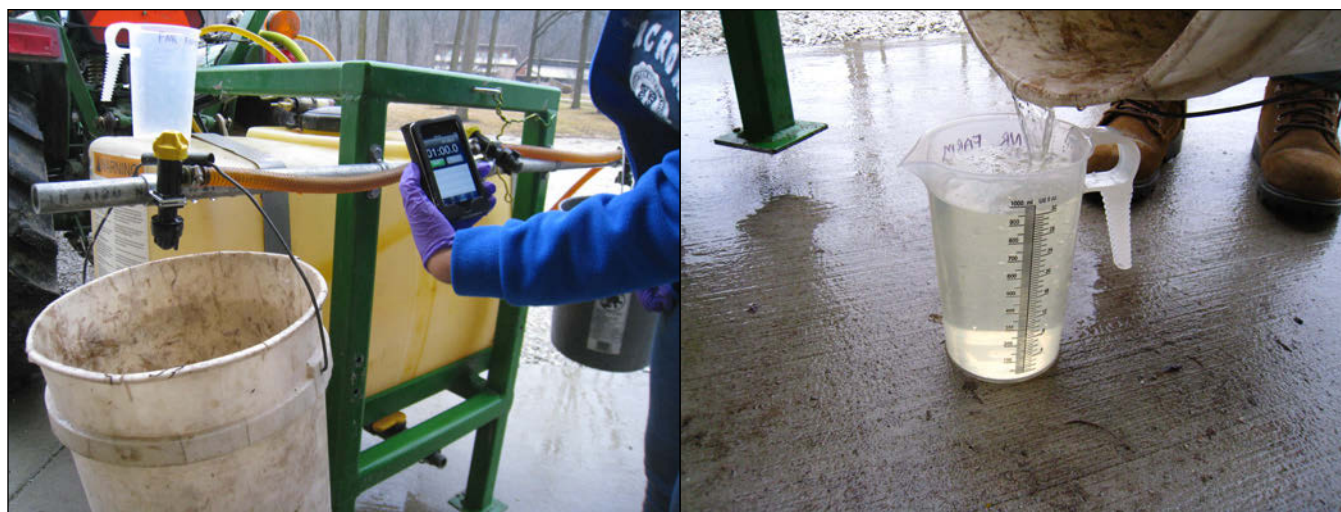
Figure 4.—Measuring amount of herbicide discharged from a flat fan nozzle for a minute as part of calibration to determine area covered when tractor is driven 3 to 4 miles per hour. (Photos by James R. McKenna, U.S. Forest Service)
