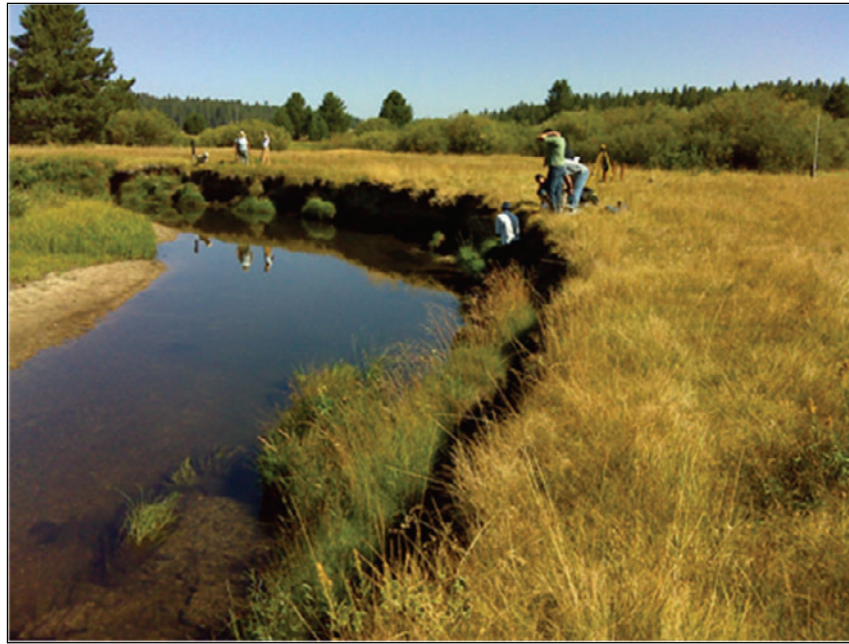
Figure 5. Measuring toppled banks along a forest meadow stream in the lower reaches of the Upper Truckee River, California (source: W. Elliot).
