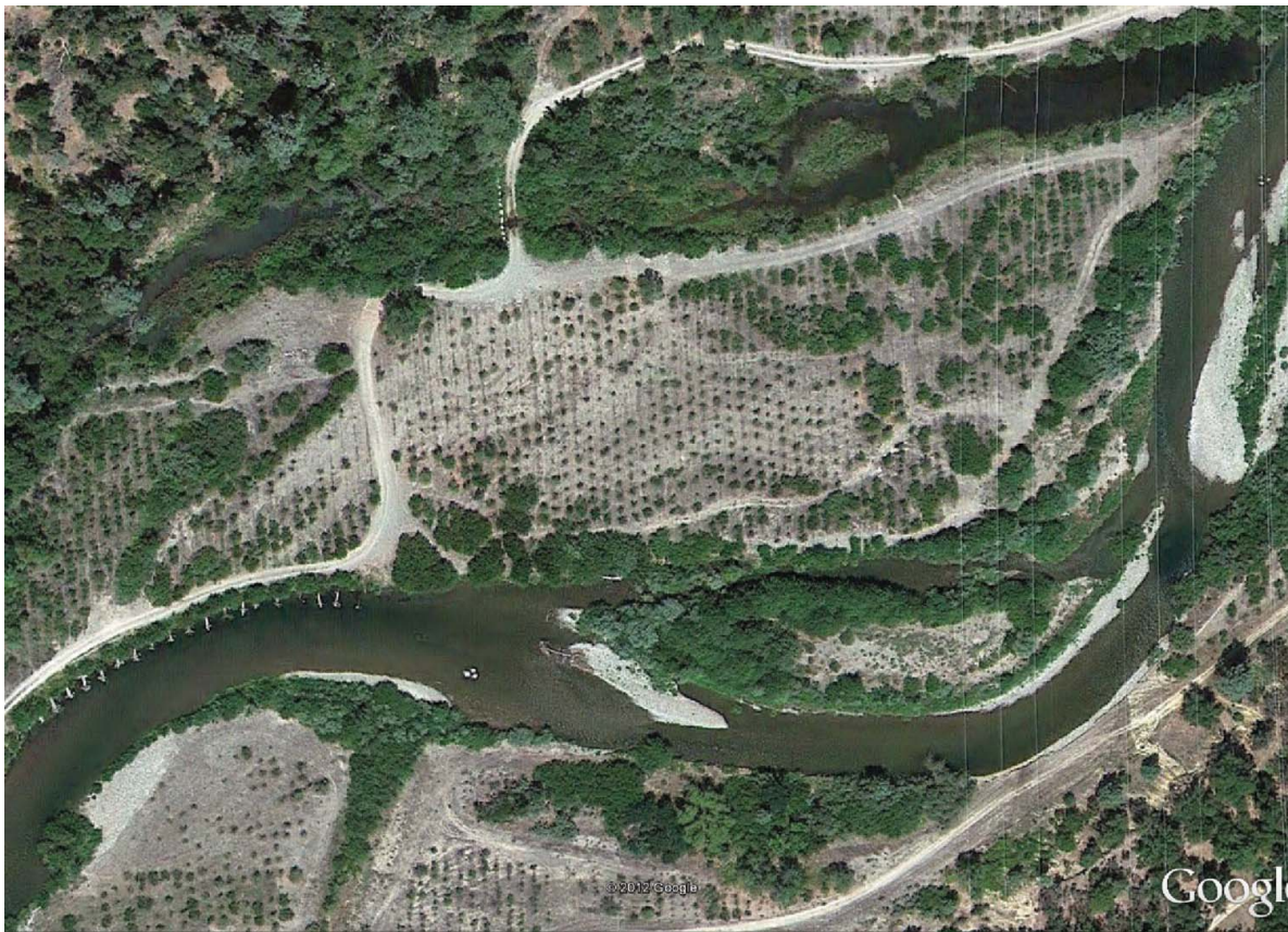
FIGURE 1. RESTO (Lower Clear Creek Flood Plain Restoration Project site 3A). This 2011 image (obtained from Google Earth) shows features of the 2002 restoration work: a wider and more sinuous channel, log structures for stability and habitat complexity in the bend at lower left, widespread spawning gravel, and a recontoured and replanted floodplain. [Figure available in color online.]
