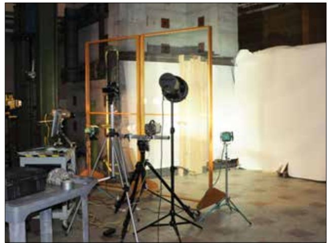
Figure 8. Configuration 4—CLT panel with high-speed photography.
