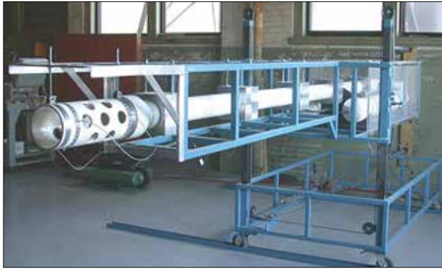
Figure 3. Debris launcher housed in the mobile firing platform.
