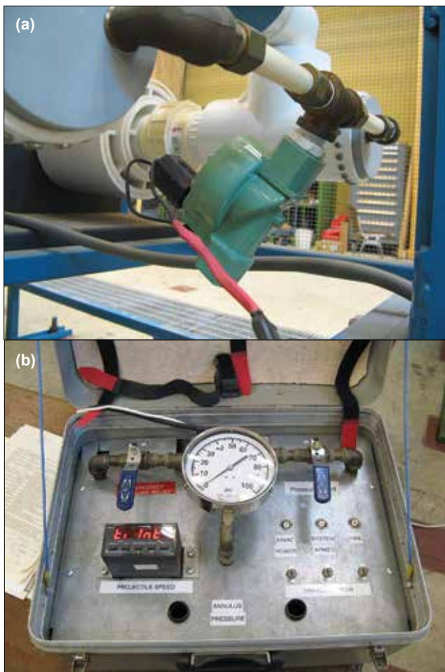
Figure 5. Debris launcher's (a) control valve and (b) instrument panel.
