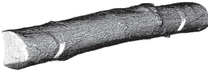
Figure 1.—Sample dot cloud image of a 3D laser-scanned red oak log.
