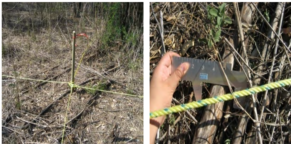
Image 1— Left: Sampling lines established in the field for carrying out the forest fuel inventory. Right: Calipers used for measuring fuel material intercepted by the sampling line.
