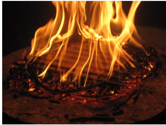
Figure 4. Crib with l/b = 48 burning from the outside edges inward.
