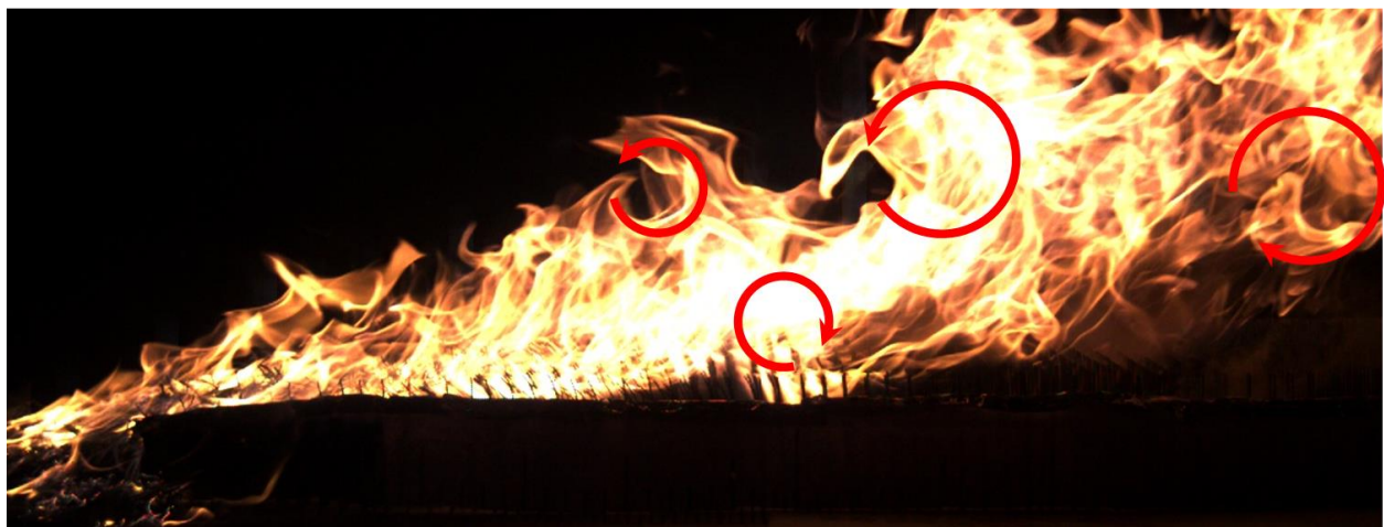
Figure 3. Flame structure normal to spread direction showing rotation of flame eddies.
