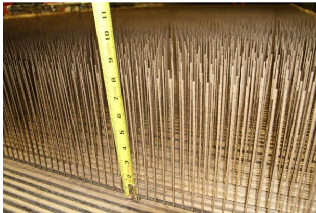
Figure 1. Picture of laser-cut cardboard laboratory fuel bed.
