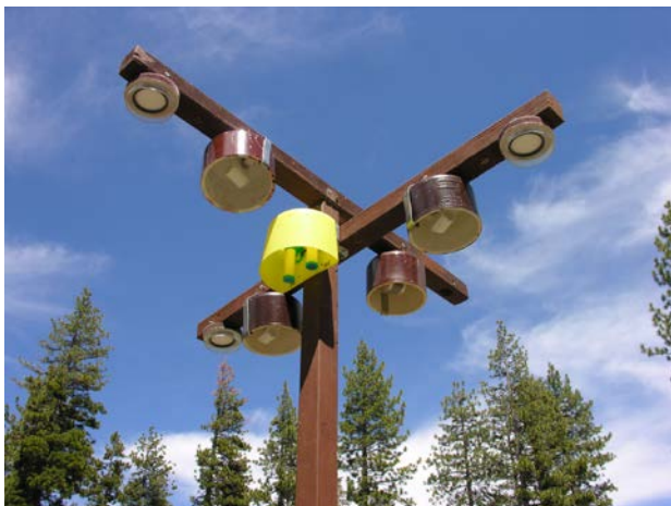
Figure 4-2. Passive sampler assembly used at 34 monitoring sites inside and outside of the Lake Tahoe Basin.
