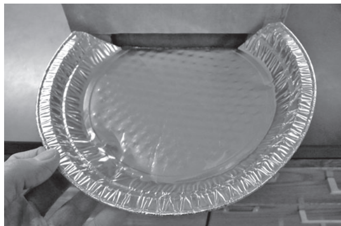
Figure 16. Aluminum pie pan cut to form a hand held feeder to place seeds into the seed chute of the box aspirator.
