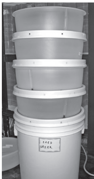
Figure 2. Pressurized seed dryer using bucket sized paint strainer.
