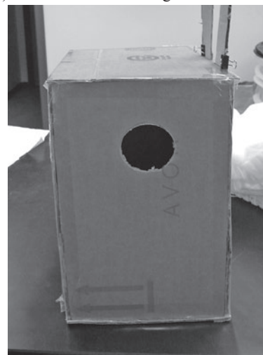
Figure 12. Vacuum source connection for 2 inch (5.1 cm) pipe on the box aspirator.
